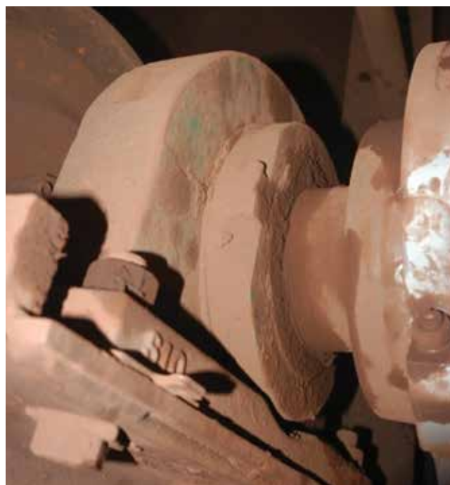
Fig. 20. Timken Split Cylindrical Roller Bearing Housed Unit is shown here in a steel industry application.
